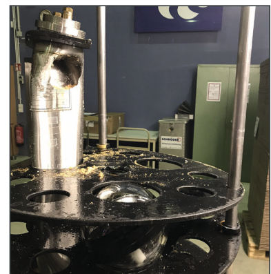
Titanium pressure vessel with a rated depth of 600 bar failed at 574 bar. VITROVEX 7.5" glass instrumentation sphere with LED lights for video recorder in close proximity of the Titanium pressure vessel was not compromised by the implosion shock wave.
