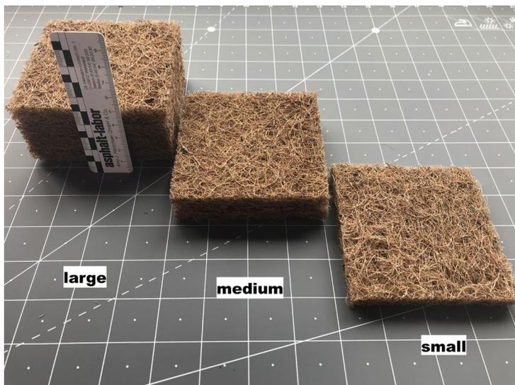
All fibre pads are square shaped (100mmx100mm), only the height is different.
